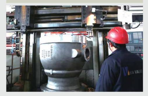
valve integrity Viza uses high-pressure gas instead of water as a medium in the shell test. Since gas molecules are smaller than water, they will reveal potential problems more easily than is the case with hydraulic testing. With the valve immersed in water, any gas bubbles in the water will reveal the presence of pinholes in the valve body.
