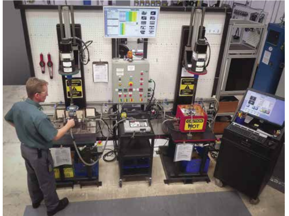
Alexander Kraus, Lab Technician, performing an API 624 test at one of Velan’s R&D labs located in Granby, Quebec, Canada.
