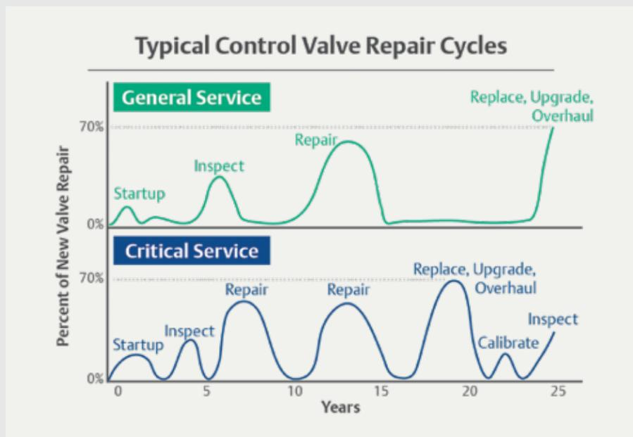
Figure 1: Valves will require varying types of services at dissimilar intervals depending on the service.
