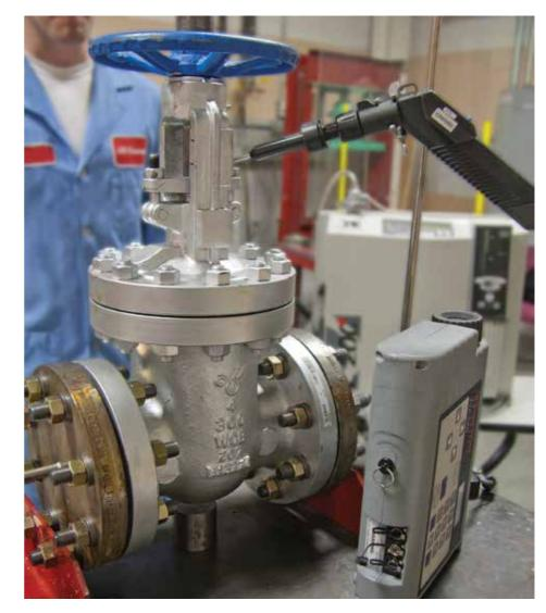
use are working at the highest level of efficiency and functionality. The investment in on-site testing allows Chesterton to work with OEM valve manufacturers' to test various types of valves, sizes and pressure classes. Not only does Chesterton test to current and future standards like the API 624, API 641, but also to troubleshoot or replicate what may have occurred in the field.
