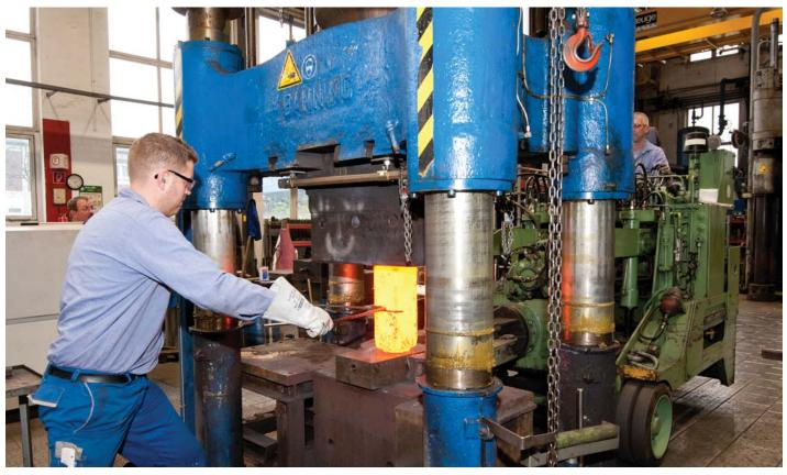
Forged stainless steel is a common material for BASF's high pressure valves. Courtesy BASF SE.
