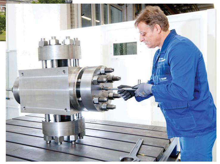
When fully assembled, BASF's high pressure valves can weigh anything up to 2½ tons. Courtesy BASF SE.
